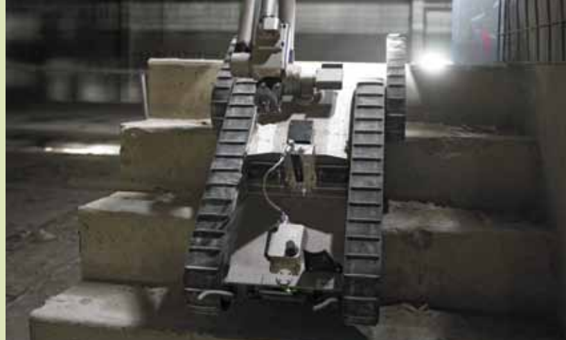
The iRobot® 510 PackBot® with User Assist Package (UAP) includes retro-traverse, self-righting and heading hold, semi-autonomous capabilities that improve mission success.
