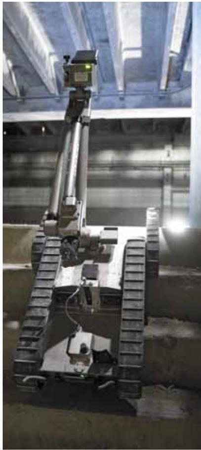
*The iRobot® 510 PackBot® with User Assist Package (UAP) includes retro-traverse, self-righting and heading hold, semi-autonomous capabilities that improve mission success.*
