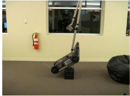
Fig. 7. MTC-based weight shifting controller moves arm forward to allow PackBot to climb over obstacle without rolling over backwards.
