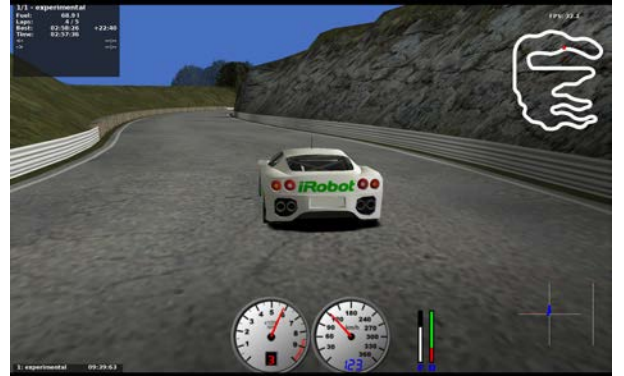
Fig. 3. MTC DSC controller driving simulated Ferrari 360 Modena in TORCS on a twisting alpine road course. The inset at the top right corner of the screen shows the track layout, and the red dot on the track represents the vehicle's current position.
