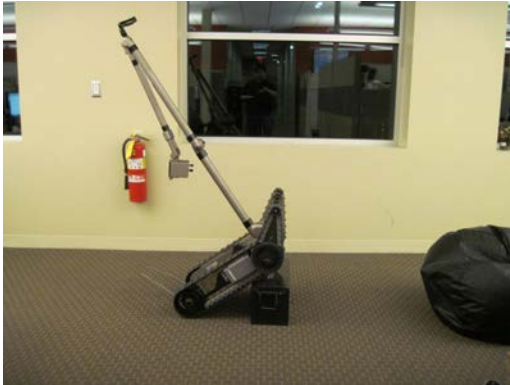
Fig. 6. PackBot attempts to climb obstacle with shoulder joint in vertical orientation ( 90^\circ ).
