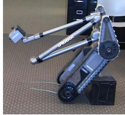
Fig. 4. PackBot attempts to climb obstacle and starts to roll over backwards.
